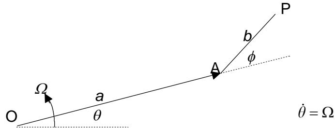
Acceleration of A perpendicular to AP is  $a\Omega^2 \sin \phi$
