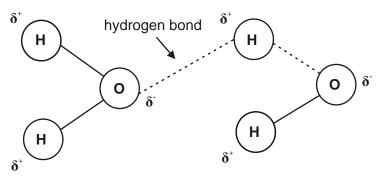
1 hydrogen bond represented as, horizontal / vertical, dashed line between O on one molecule and H on the adjacent molecule;
