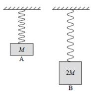
The objects are given identical vertical displacements from their equilibrium positions and then released. Air resistance may be neglected.
