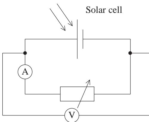
The student keeps the intensity and wavelength of the incident light constant and adjusts the variable resistor to obtain the following set of results.
