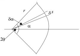
If the framework can be in equilibrium with any part of the semicircle in contact with the floor then the centre of mass of the framework must be directly above this point of contact hence at centre of semicircular arc.
