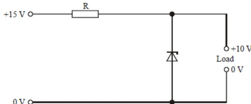
The maximum output current supplied to the load is 100 mA. The zener diode must have a minimum current of 10 mA passing through it to maintain its voltage.
